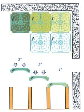
The arrows on the domes should always indicate the direction in which the installation operator looks.
