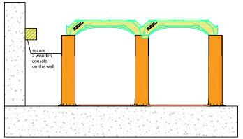
2) Cut the dome at the exact size to close the opening and place it on the pipe and the console.
