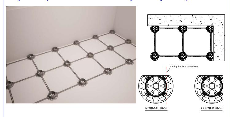
**2.** Press the PVC pipes that have been cut according to the project firmly into the base slots.
