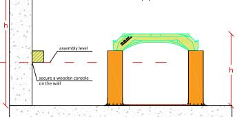
2) Cut the connecting piece at the dome and place the dome on the wooden console.
