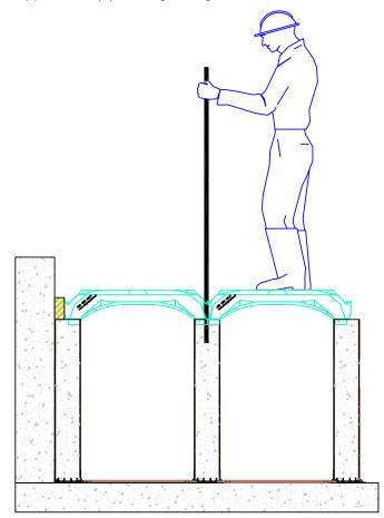
Use a vibrator when pouring the concrete of the slab on top of the domes, making sure that the concrete is fully spread and settled.
