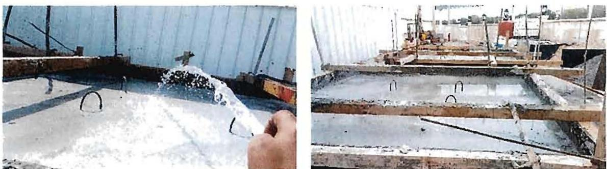
Figure 4: water curing the slab samples.
