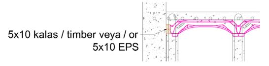
2.5. At the wall finished, where the last row of domes is longer than the distance to the wall so as not to place a new row of domes, the domes must be cut at the full wall distance and placed on the wooden consoles fixed to the wall at the appropriate height as the other domes on PVC pipes.
