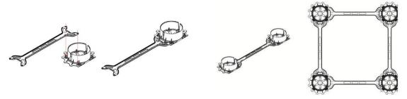
When used in all directions, a maximum 4 spacer are required per m<sup>2</sup>. However, with respect to the application geometry, it is also possible to connect all the spacers in one direction and to skip 2 or 3 in the other 90-degree direction. For example;
