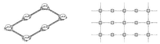
At less than 100 cm heights spacers could be completely omitted except at starting points or around columns etc. assuming a standard wet concrete pressure will be applied. Also, in ramp applications, the spacers cannot be used in the direction of the inclination.
